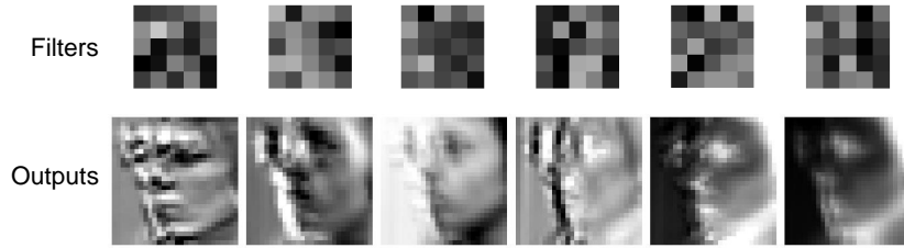
Fig. 3. Some trained filters and their outputs of an input image in the first convolutional layer. The sizes of filters and the outputs are 5 \times 5 and 28 \times 28 pixels respectively.
